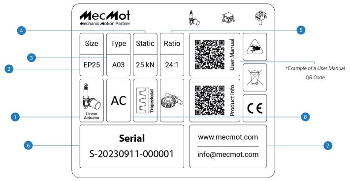
\*Example of MecMot Linear Actuator Rating Plate
