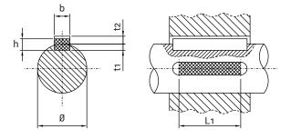
Material: C45 (1.1191) according to EN 10083-1 Load type: Drive - Uniform / Load - Light knocks
