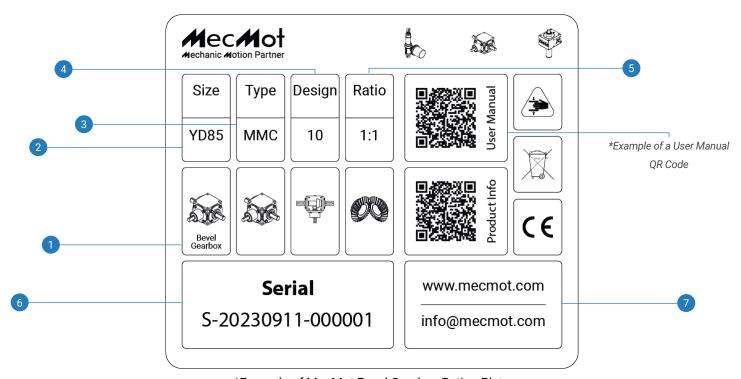
\*Example of MecMot Bevel Gearbox Rating Plate
