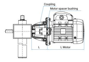
In general, it is always advisable that the motors incorporate a brake, standard brakes are sufficient for each motor size in most cases. This will ensure the screw does not loose position when it stops or if there are vibrations, etc.
